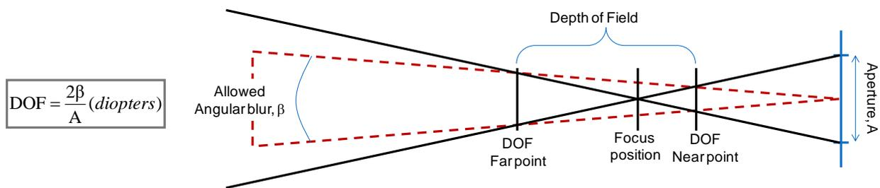
Figure 1: Diagram showing the optical system parameters that influence DOF
