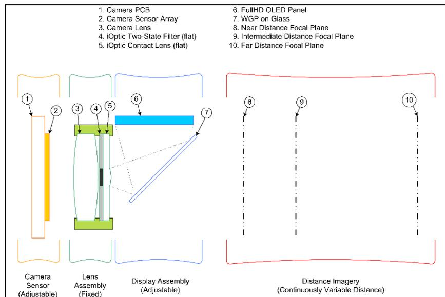
Figure 8: eMacula™ eyewear display camera simulation system
